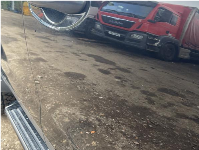
3: Door osf Poor Previous Repair Rippled UpTo 30%
